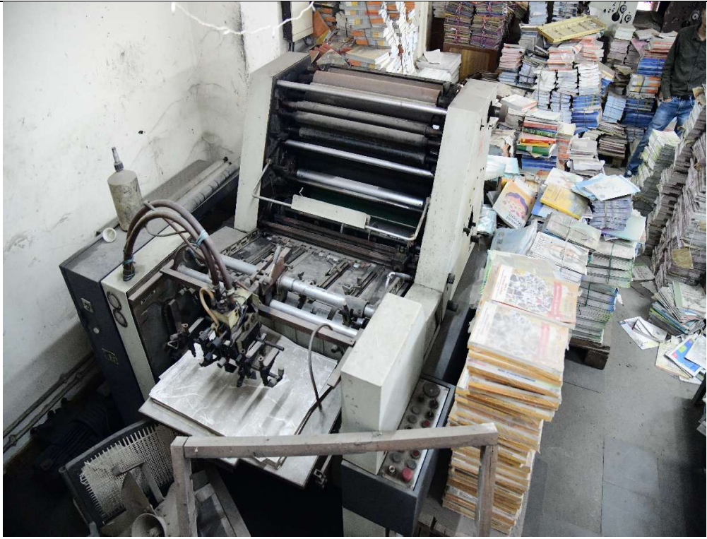
Dominant 715 Offset 1-Color Printing Machine 1 SR No 1874
