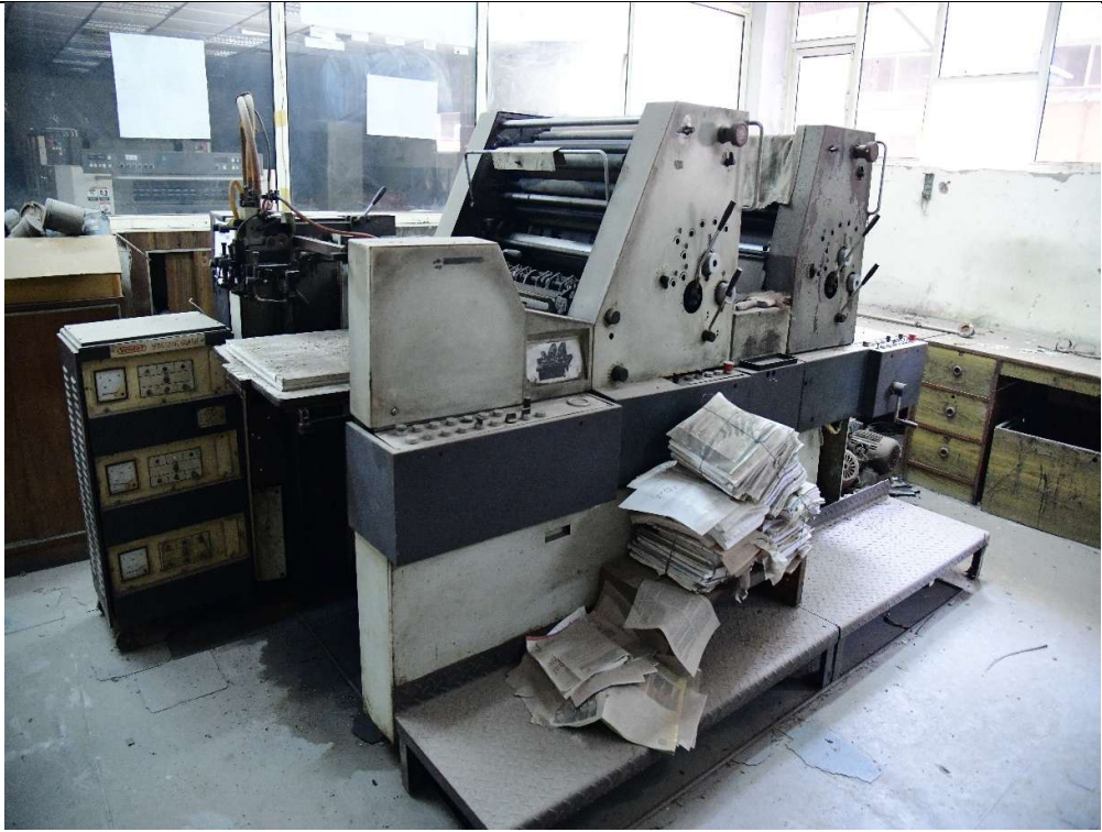
Dominant 725 2- Color Printing Machine SR No142 with Stabilizers
