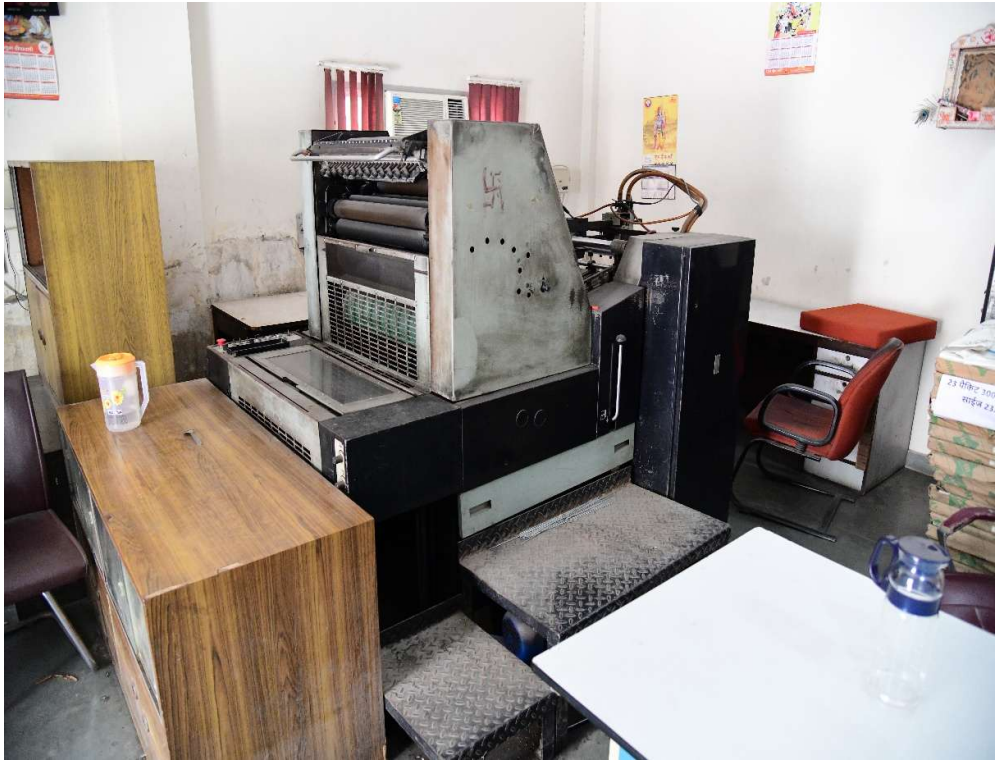
Dominant 715 Offset 1-Color Printing Machine SR No 2035
