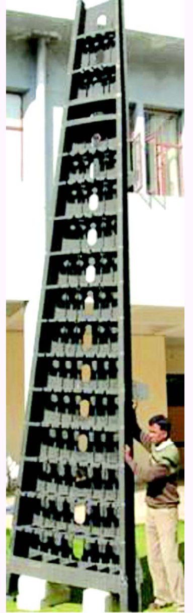
Photograph of Coinfused Cured Wing Interspar Box realised using VERITY process
