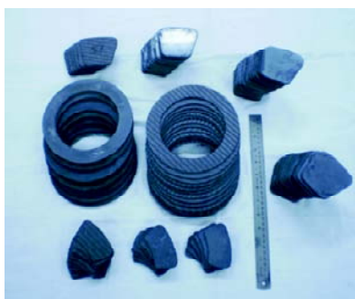
Designs of standard clutch friction plates made of carbon fibre reinforced silicon carbide
