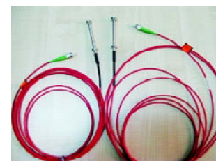
Encapsulated in specially designed SS-mount for monitoring of health of structures like bridge dam and other civil engineering structures
