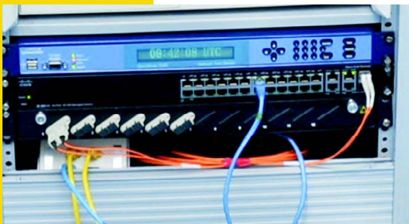
NTP server installed in the T&F Division, NPL, India
