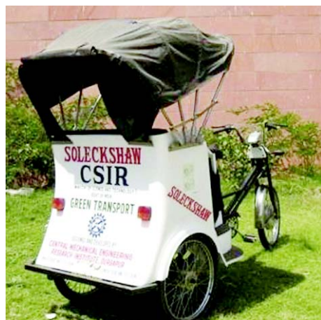
BLDC based, front wheel drive soleckshaw , prototype manufactured by CMERI, Durgapur
