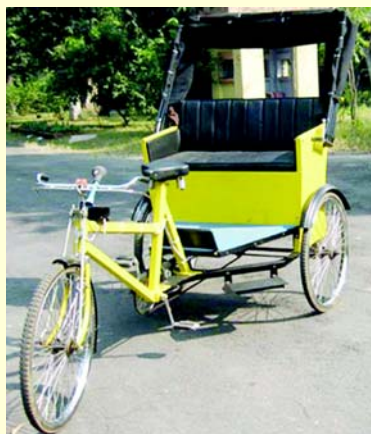
PMDC based, rear wheel drive soleckshaw , manufactured by M/s Dean Systems (one of the licensee), Kolkata
