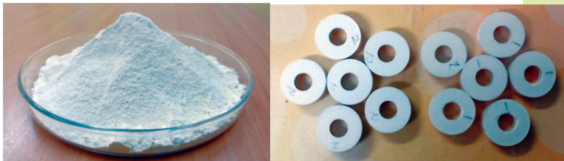
PZT powder and fabricated PZT rings prepared by the CSIR-NAL team, for accelerometer applications
