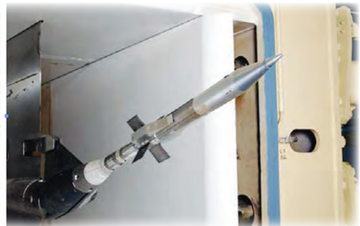
ATV model for aerodynamic force and moment measurements for unsteady pressure measurements
