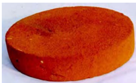
Making of Terafil discs — The innovative water filter designed by CSIR scientists
