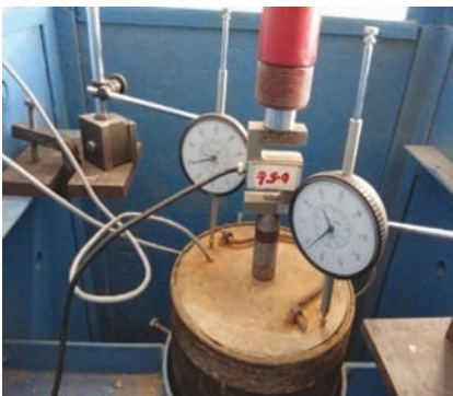
Fig. 4. View of complete load test set-up
