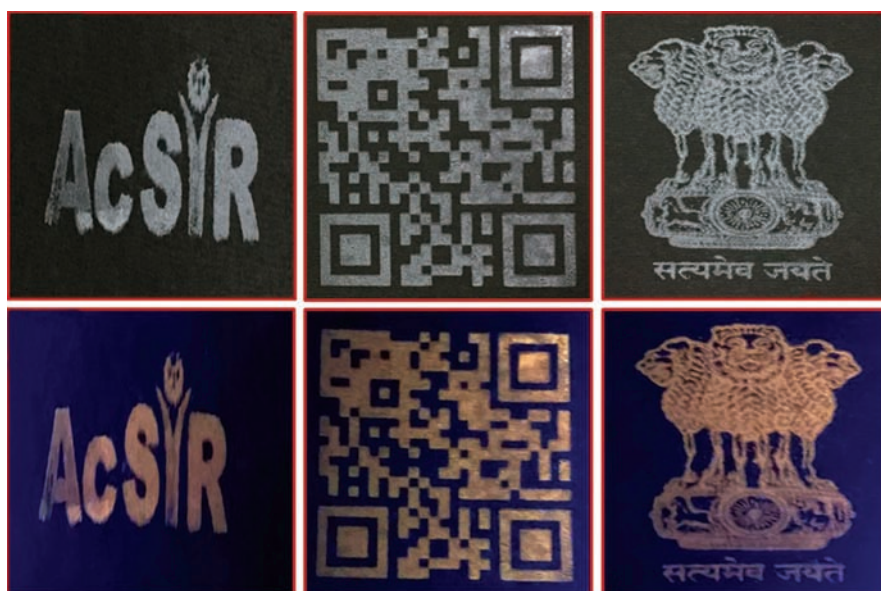
Prints using the new security ink appear differently under normal light (a) and under UV light (b)
