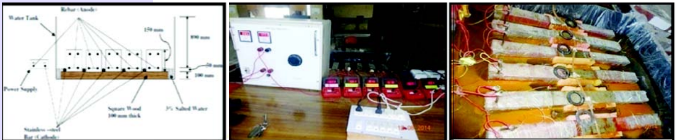
Fig. 2: Scheme for corrosion acceleration and beams corrosion in progress
