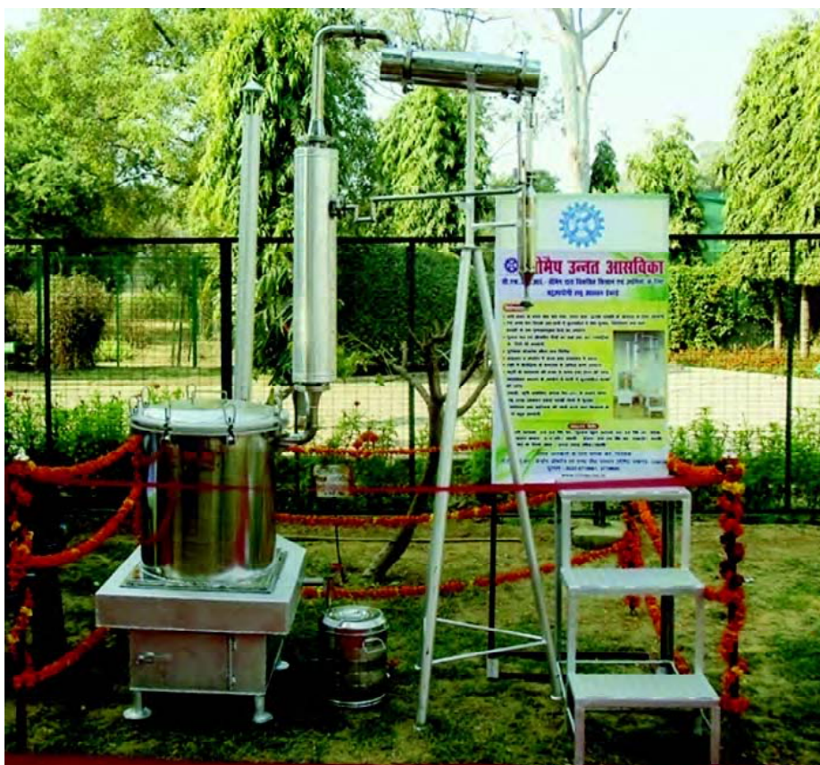
CSIR-CIMAP Unnat Asvika, a multi-utility portable distillation unit released on the occasion
