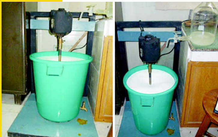
Fig. 1. Set up for bench scale preparation of silica nanoparticles
