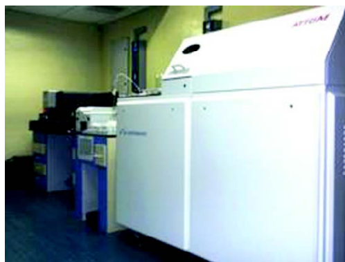
Laser Ablation, Desolvating Nebulizer unit, autosampler (L to R) and HR-ICP-MS systems inside the Lab
