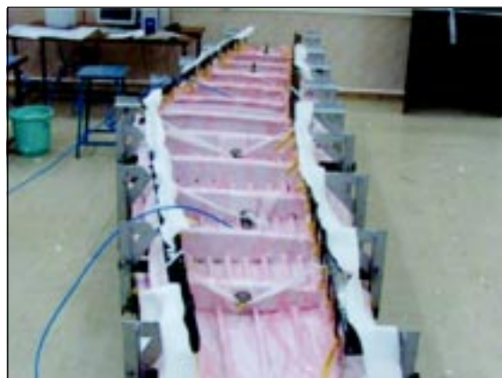
Part bagged before the autoclave
