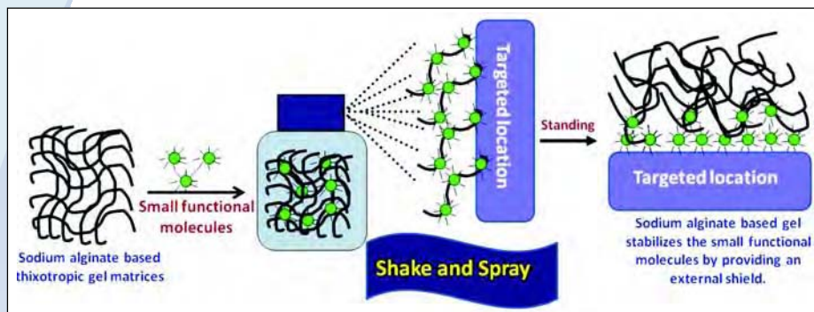
Fig. 3. Schematic representation of the alginate acid amide based sprayable gel delivering active molecules
