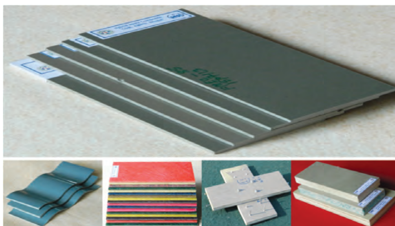
High-performance hybrid composite materials based on fly ash and natural fibre developed by CSIR-AMPRI Bhopal
