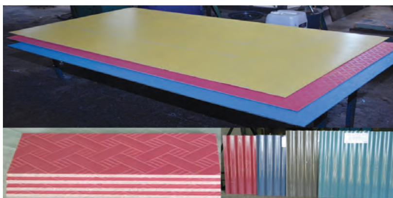
Wood substitute hybrid composite materials based on fly ash/red mud/marble wastes reinforced with natural fibres developed by CSIR-AMPRI
