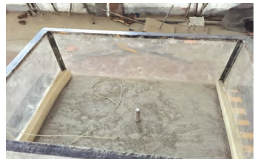
Fig. 2: (b) Use of Foam to Nullify Boundary Effects
