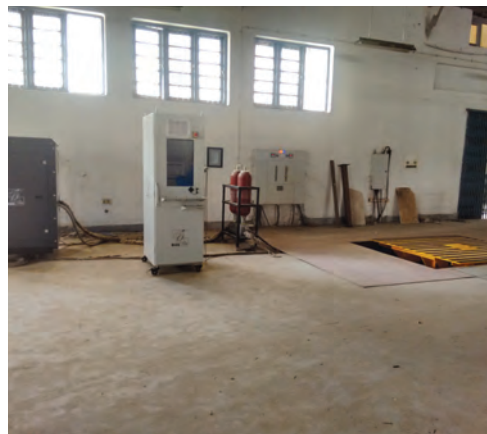
Fig. 1: Uni-Axial Shake Table & its Accessories
