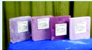
Al-foam filled bracket for noise and vibration attenuation
