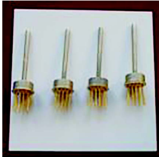
Fig. 4: Pressure sensor packaging on TO- headers
