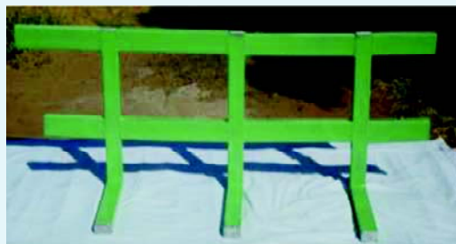
Al-foam filled bracket for noise and vibration attenuation
