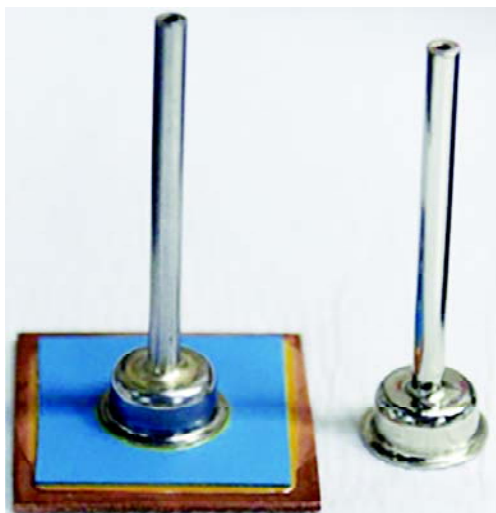
Fig. 3: Pressure sensor packaging on LTCC
