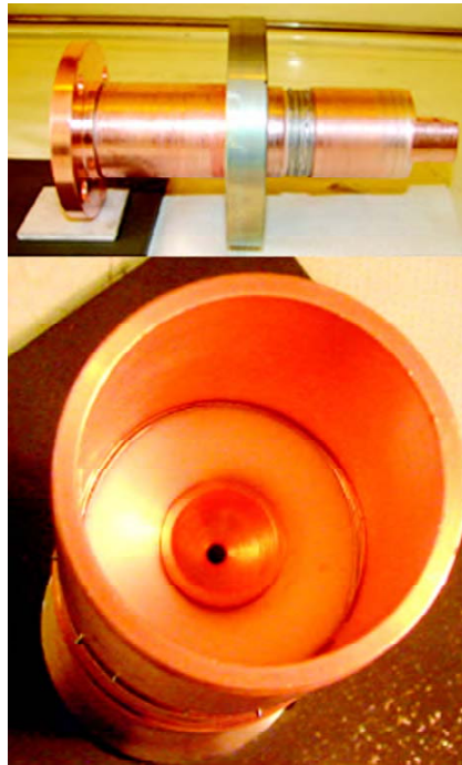
Fig. 1: Uncooled coupler with its ceramic window
