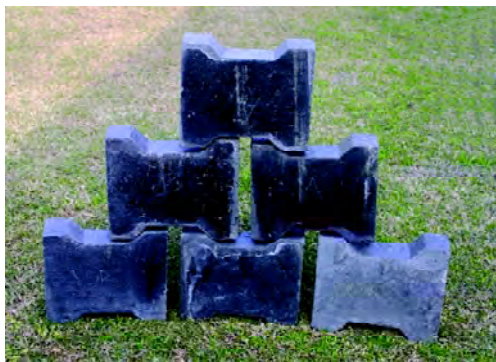
Fig 1: Two layered interlocking paving prepared from recycled aggregate
