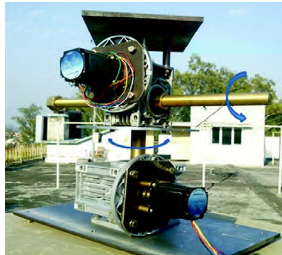
Fig. 1. Fabricated Solar Tracker without cover
