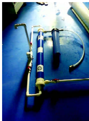
Water Purification through Ultra Filtration at H.N. Bahuguna Base Hospital, Srinagar, Uttarakhand
