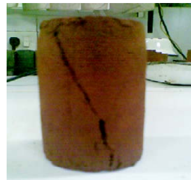
Fig. 3: Failure Pattern of Red Mud with 8% Cement
