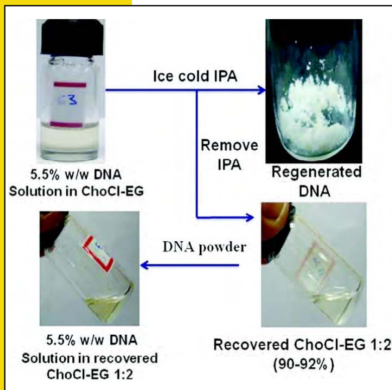
Fig. 2. Dissolution of DNA in deep eutectic solvents, recyclability and reusability of the solvent
