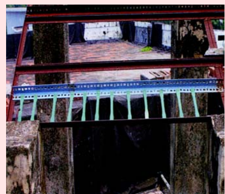
Outdoor exposed PP random copolymer in rack as per ASTM D 1435
