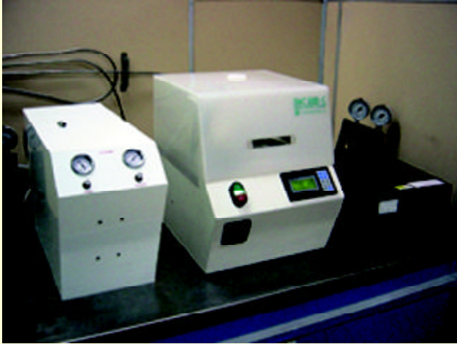
Megasonic Cleaner: 1 MHz Spin Cleaning
