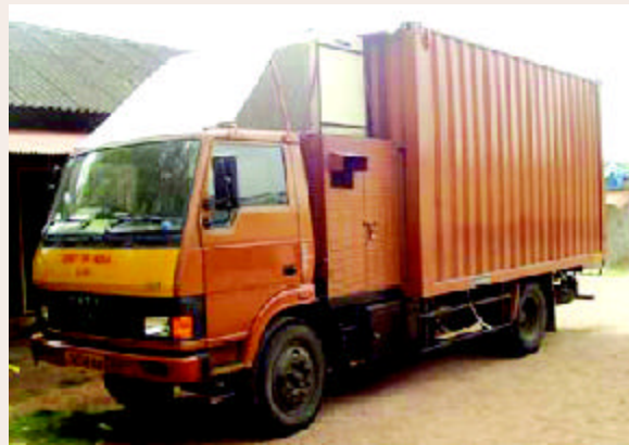
CLRI designed and tested Mobile Blast Chilling System for preservation of hides and skins
