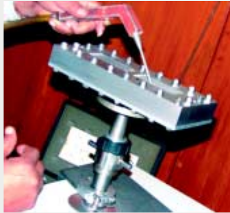
Fig. 2: Leak Testing of Brazed Window
