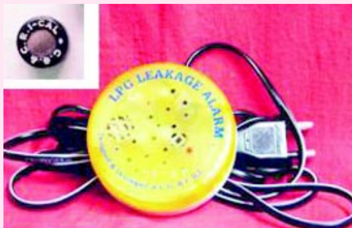
LPG/CNG Gas Leakage Alarm (Inset: Sensor Head) developed at CGCRI, Kolkata
