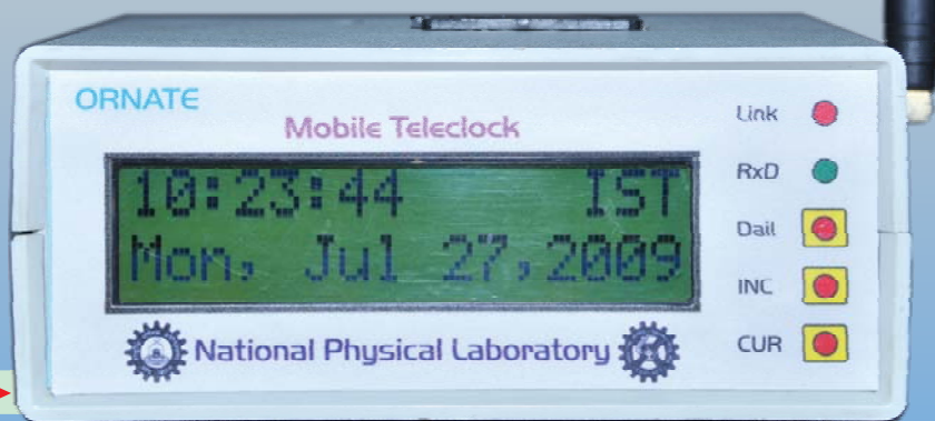
Prototype Mobile Teleclock receiver developed at NPL ▶
