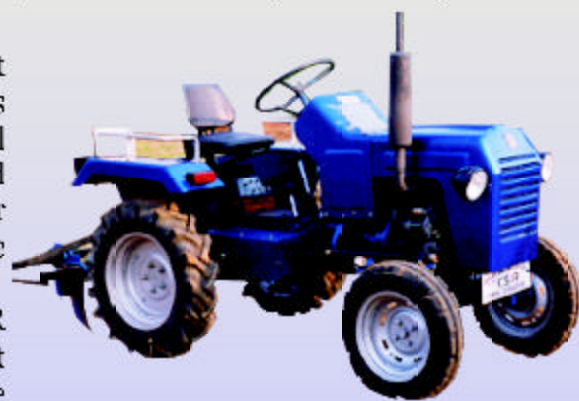
Krishi Shakti, a 10 hp tractor designed and developed by CMERI
