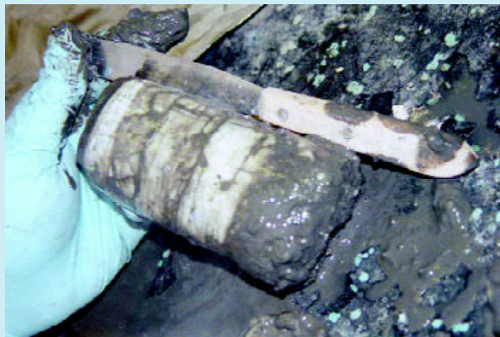
A typical gas hydrate sample from Krishna Godavari Basin
