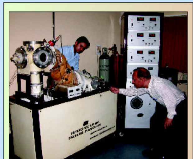
A view of the custom designed and indigenously developed S bend FCVA system at NPL
