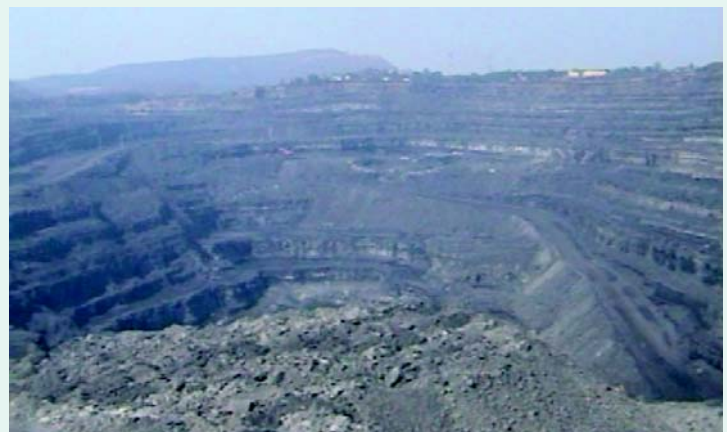
Fig. 4 : View of 15 working benches of both Coal and OB of Quarry-SEB of M/s Tata Steel Limited (TSL), West Bokaro where CIMFR-designed highwall mining would start shortly
