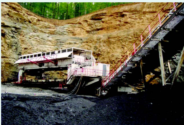
Fig. 3 : ADDCAR Highwall Mining in operation at Miller Brothers Coal LLC, Kentucky, USA
