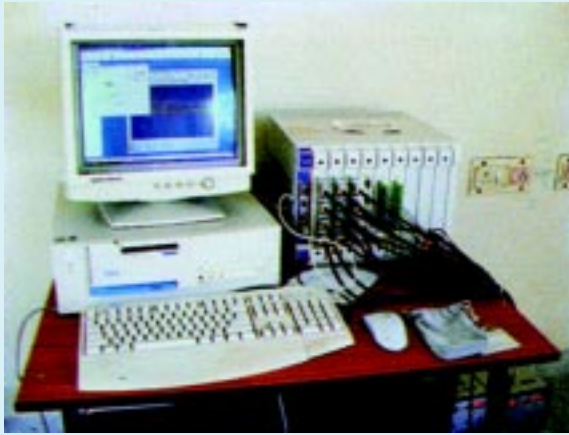
Fig. 6 — Operational wind turbine load measurements using a new portable 32-channel data acquisition system
