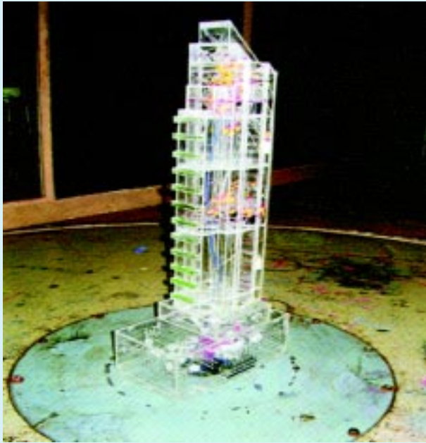
Fig. 3 — View of the model in wind tunnel
