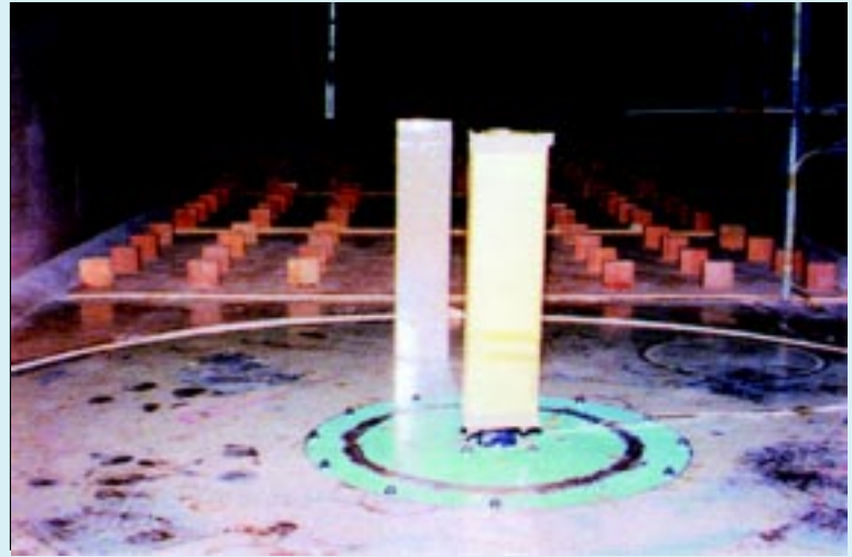
Fig. 5 — Experimental studies on across wind spectrum on a tall square building including interference
