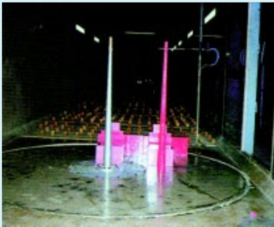
Fig. 1 – Wind tunnel experiments on chimneys and cooling towers
