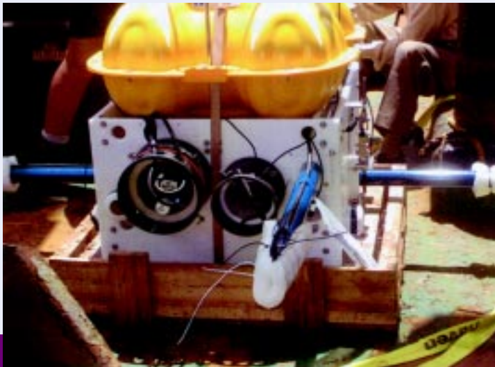
Marine Magnetotelluric equipment being assembled in the vessel
