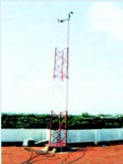
Fig. 7 — A roof top tubular lattice tower and a 3D-frame with angle sections under study
