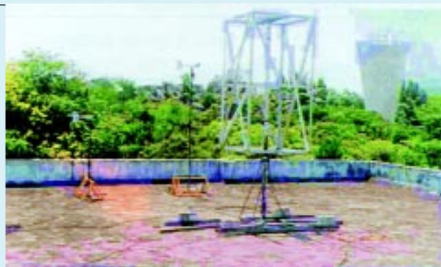
Fig. 7 — A roof top tubular lattice tower and a 3D-frame with angle sections under study
