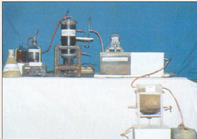
Bench scale unit for treatment of wastewater containing high organics
