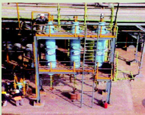
Aerial view of a pilot plant for bio-deodorization of industrial emissions containing pyridine at M/s Jubilant Organosys Limited, Bharatiyagram (U.P.)
