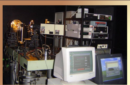
A view of the set-up for primary standard of optical radiation
