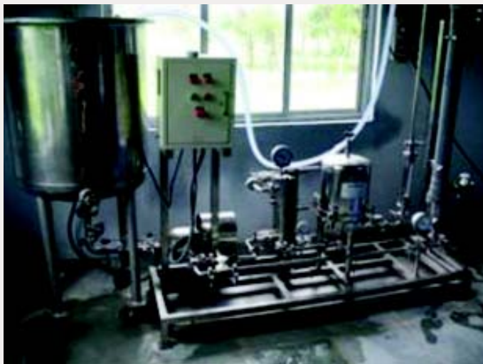
Neera filtration plant installed at the site of Gujarat Neera Federation, Saronda
