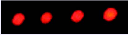
Fig. 4 : Output of Polymer-based 1x4 Optical Splitter Tested at 633 nm
