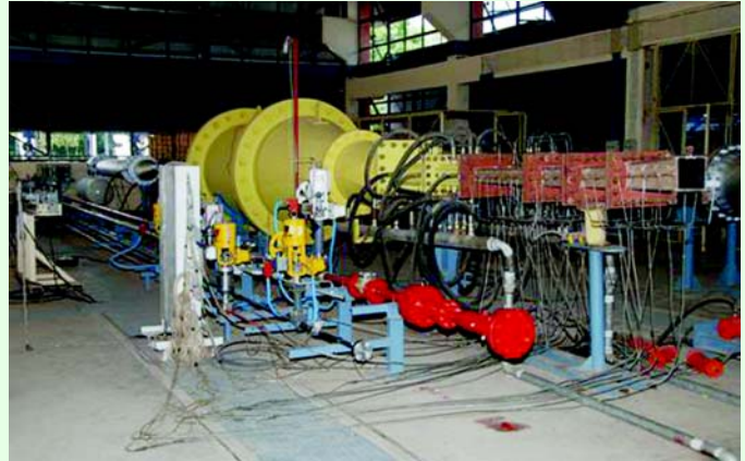
High-Speed Combustor Test Facility – Supersonic Combustion Leg
