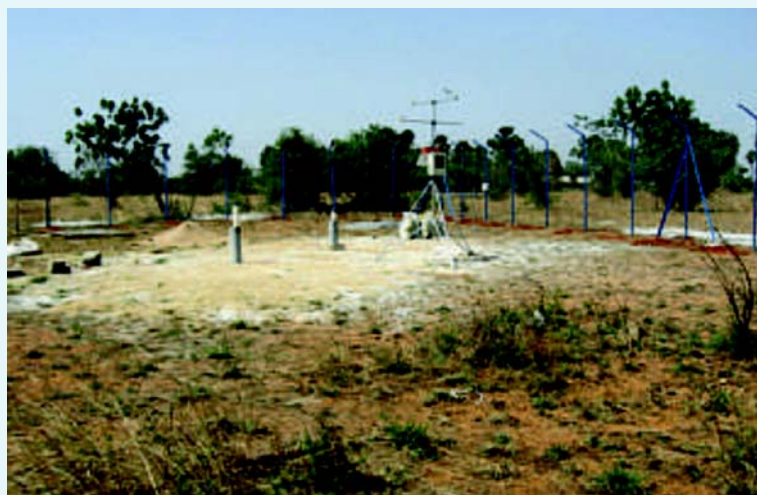
Layout of the Observatory showing automated weather station and two boreholes
