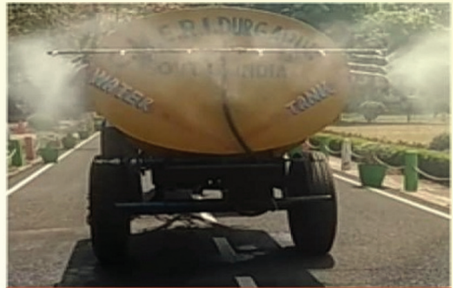
Sixteen feet span, uses 15 to 35 bars of pressure, 12 nozzles that ensure optimum radial coverage, 2000 to 5000 litres tank, 22 LPM pump.
